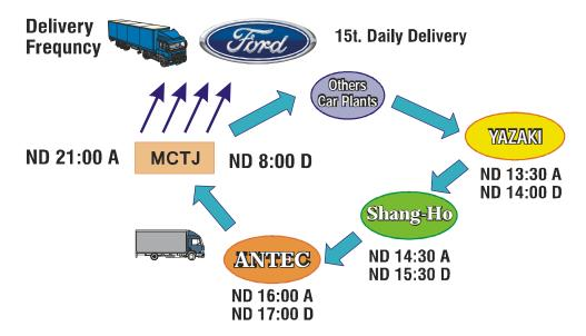
HO), whose components of the cars wiring are delivered through LLP system executing a Milk-Run process. The Milk-Run process can be seen in Figure 8:
