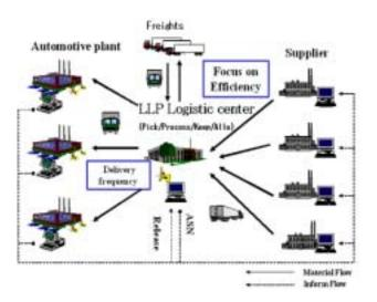
with parts suppliers is to eliminate excess parts inventory through JIT delivery. The following major process-reengineering efforts were conducted to enable logistics synchronization. First is the material requirement process driven by production scheduling of Ford Taiwan. The LOGICOM system
