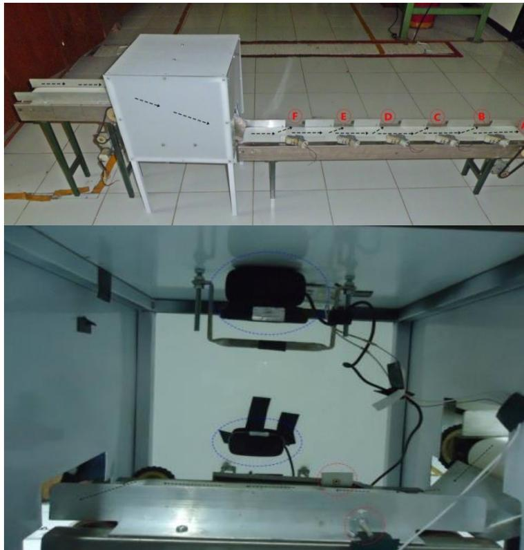
Figure 2. A typical layout for determining conveyor speed – image capturing process
