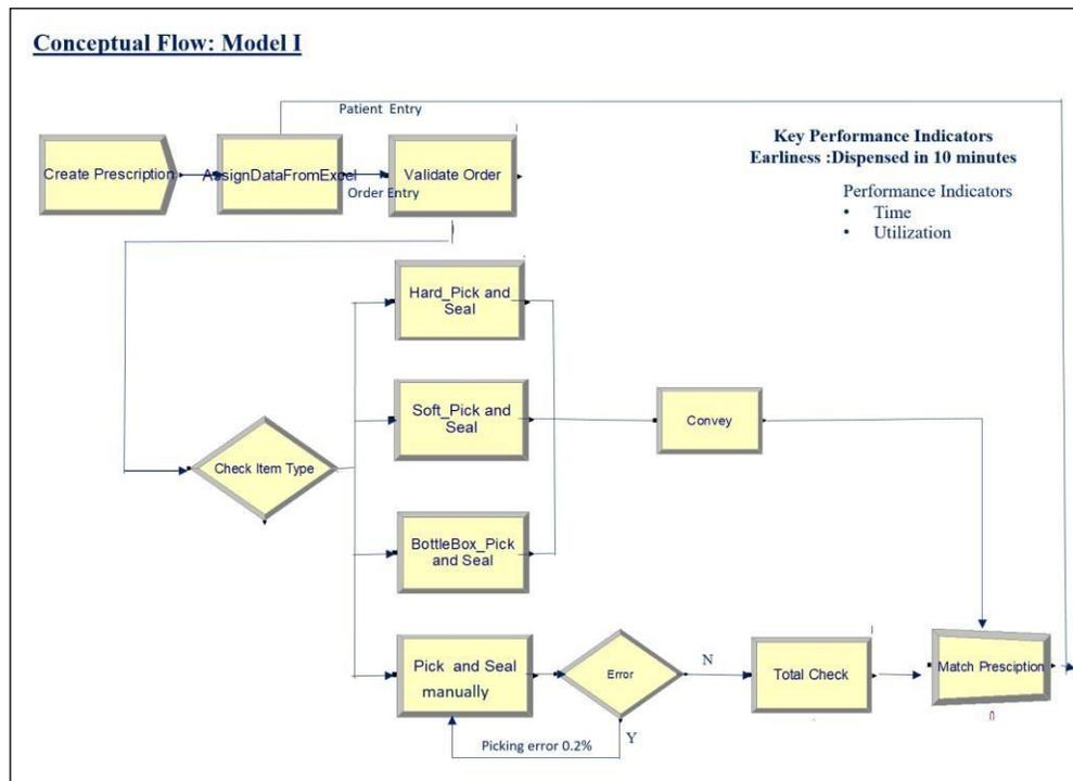
**Figure 3.** Conceptual flow of simulation modeling: Model I, Parallel triple machine
