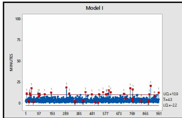
Figure 6. Display control chart of process time of model I AS-IS situation
