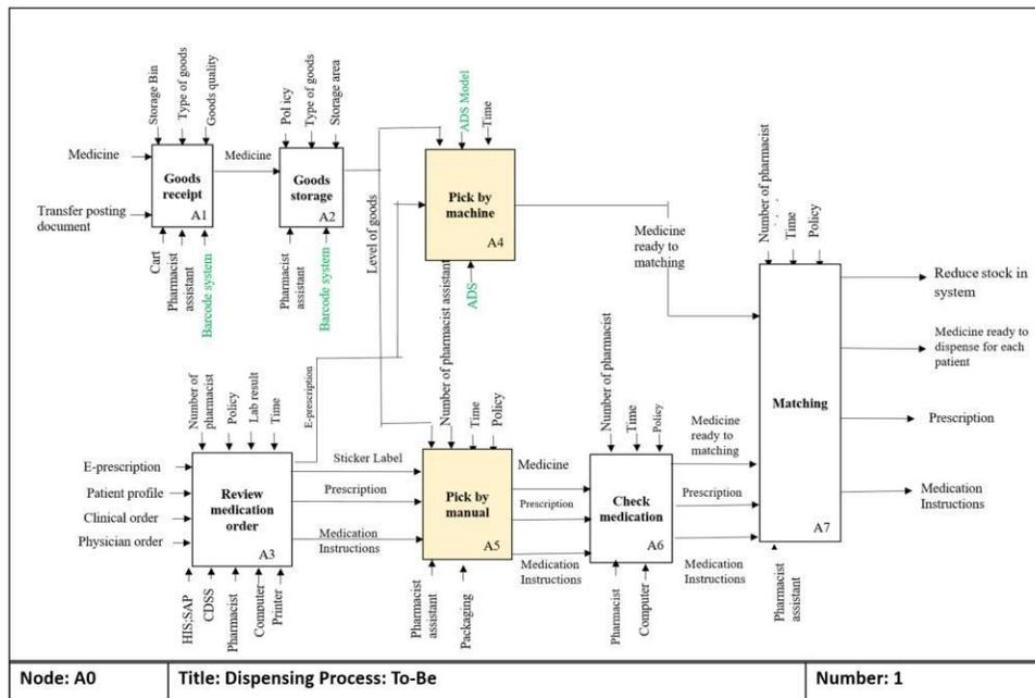
Figure 2. Dispensing process after process development
