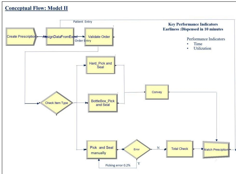
**Figure 4.** Conceptual flow of simulation modeling: Model II, Parallel double machine
