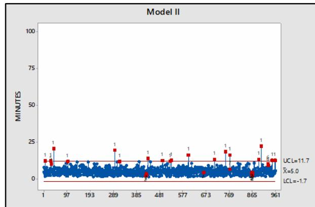
Figure 7. Display control chart of process time of model II
