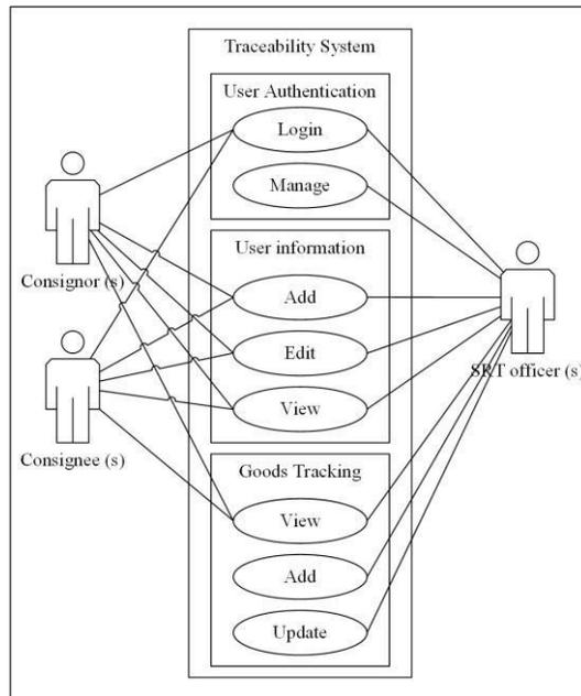
**Figure 2** Traceability System Use-Case Diagram
