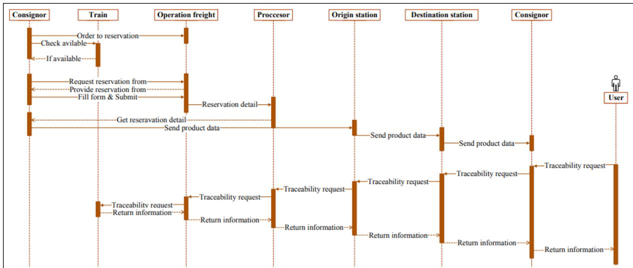
**Figure 4.** UML sequence diagram of information exchange among the actors
