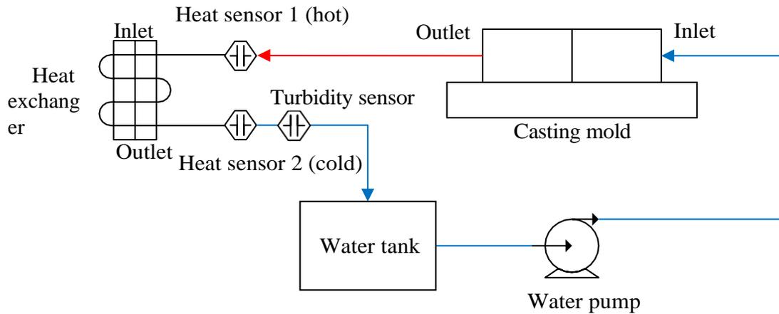
**Figure 3.** Proposed the predictive maintenance system architecture with sensor combination.
