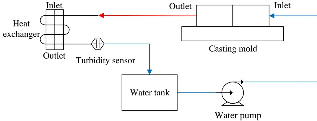
**Figure 2.** The predictive maintenance system architecture with turbidity sensors (Suryadarma et al., 2020b)
