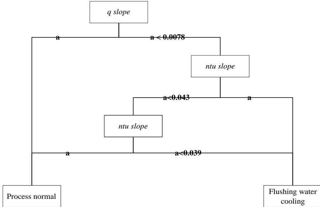
**Figure 11.** Decision structure of rule-based classification by combining slope
