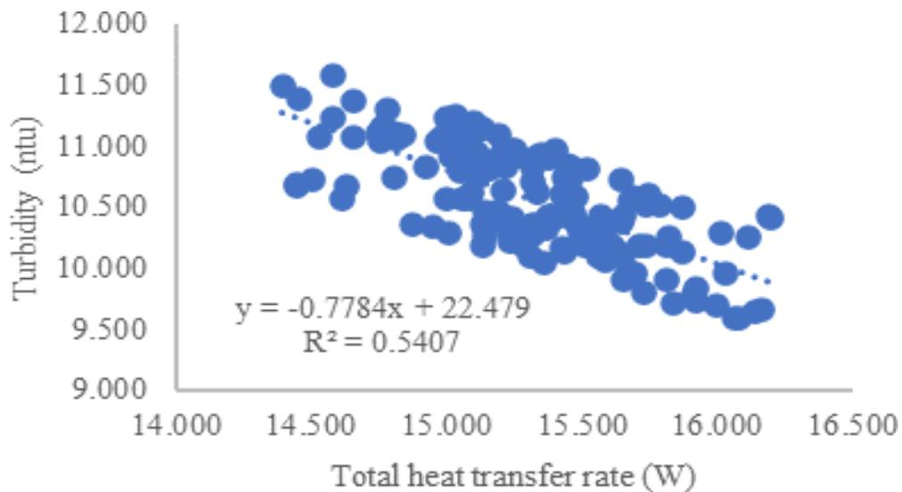
**Figure 7.** Relationship between turbidity and total heat transfer rate.
