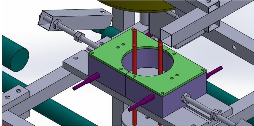
**Figure 4.** Prototype of continuous gravity die casting mold.
