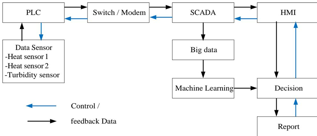
**Figure 5.** The prototype of the predictive maintenance system with sensor combination.
