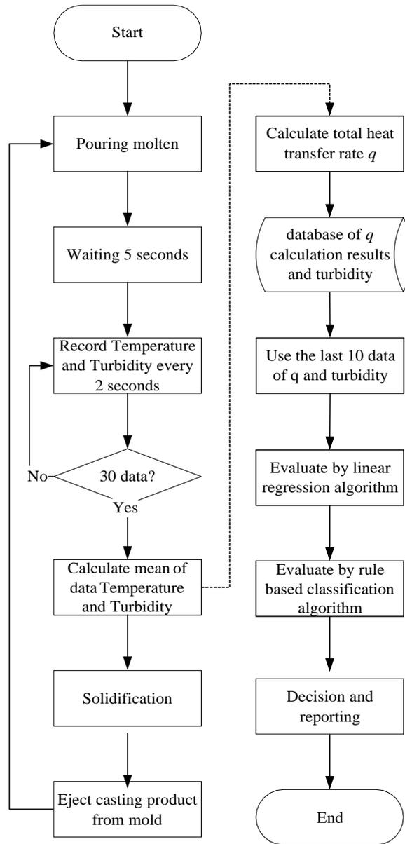
**Figure 6.** Experiment procedure.
