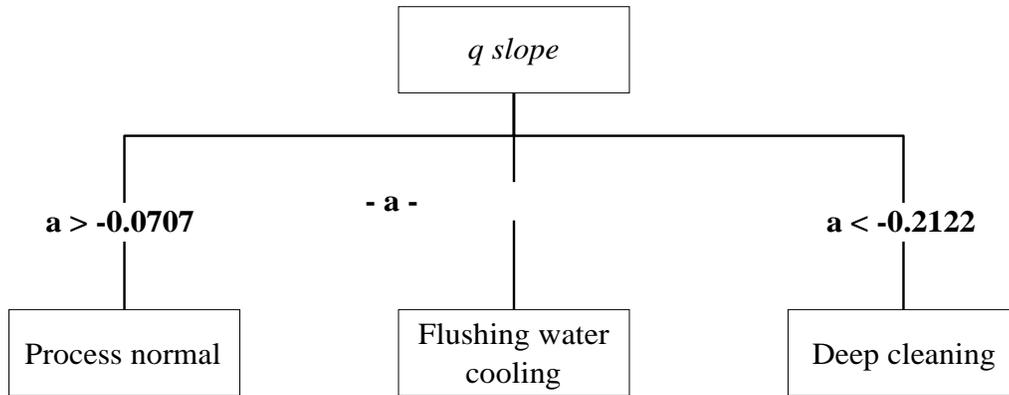
**Figure 9.** Decision structure of rule-based classification by  $q$  slope
