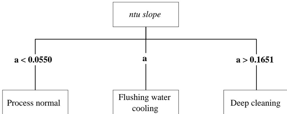
**Figure 10.** Decision structure of rule-based classification by  $NTU$  slope
