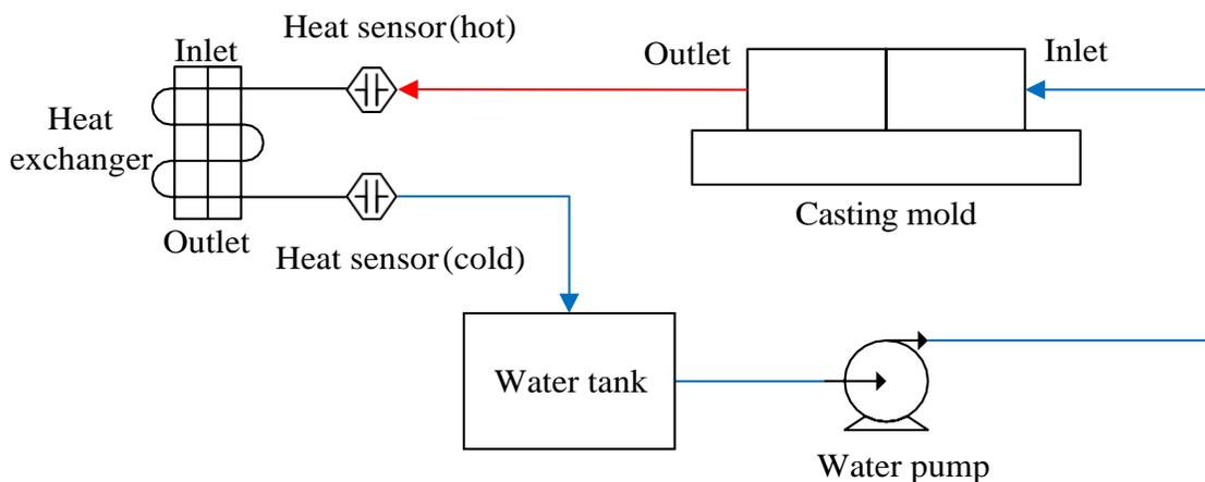
**Figure 1.** The predictive maintenance system architecture with temperature sensors (Suryadarma et al., 2020a)
