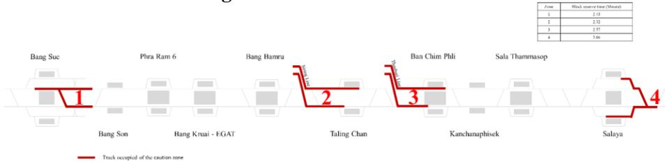
Figure 7. Occupied position of caution zone on the track
