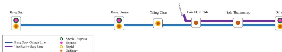
**Figure 5.** Long distance train station stop pattern
